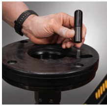
PIN PROTECTORS for centering pulling unit
