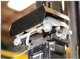
Multi-Stage Locks Lower-to-lock is standard.
